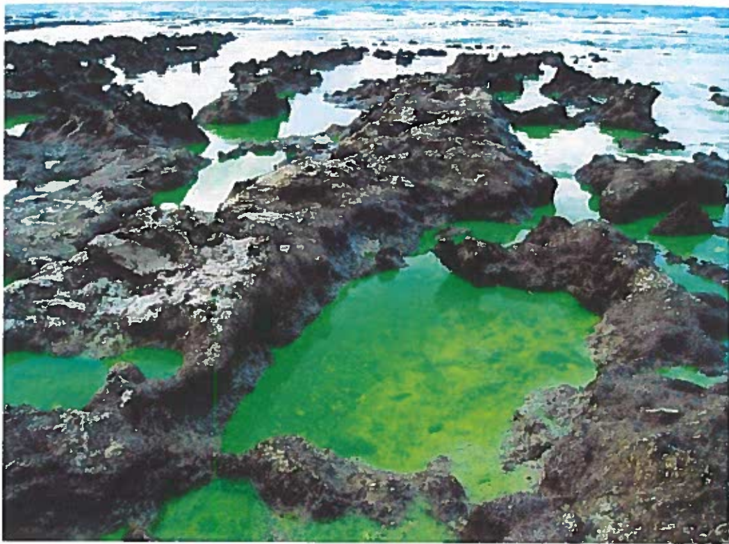
Photo 3-1. Visual identification of Fluorescein Dye at time of breakthrough, Andersen AFB, Guam.
