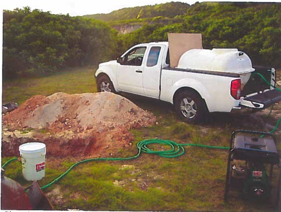
Photo 2-5. Tinopal CBS-X Dye injection at the OB Unit, Andersen AFB, Guam.
